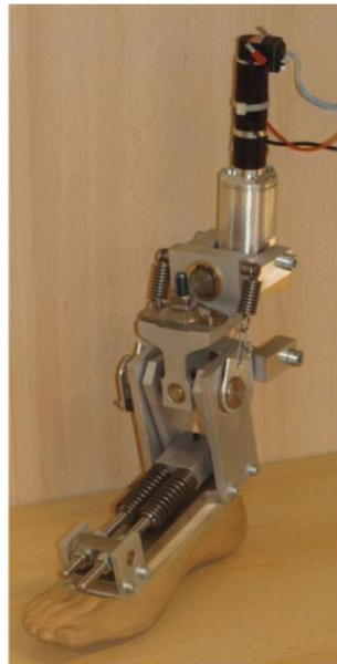
Figure 17. Ankle Prosthesis prototype developed by UCL-Belgium [1]
