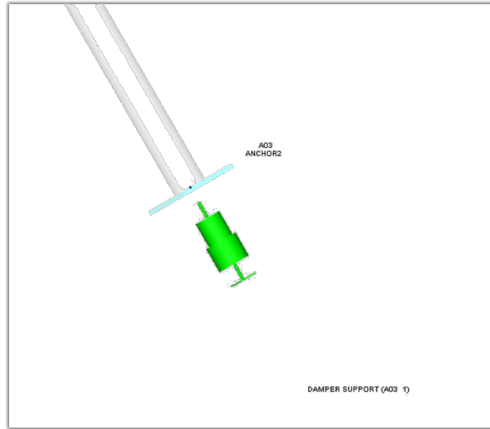
Figure 34. Zoomed portion of the bottom segment of the stress analysis model using Bentley Autopipe
